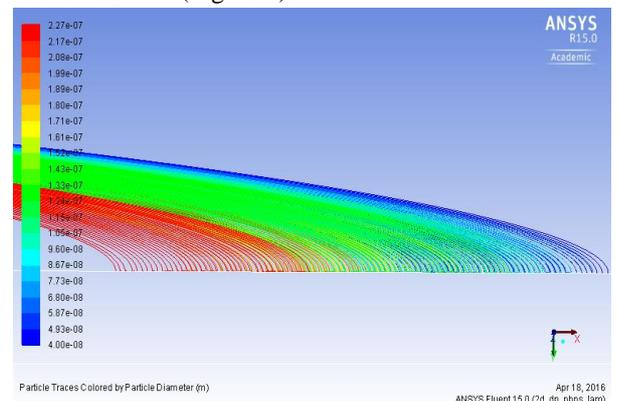
**Figure 2:** Particle displacement toward the cold wall.
