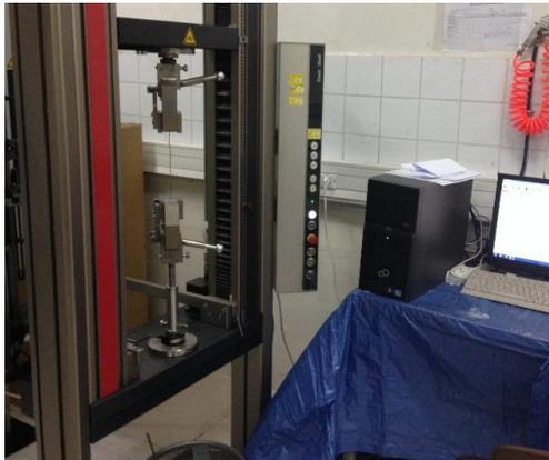
Figure 2. Machine de traction "ZWICK ROELL"
