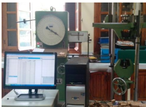
Figure.1 : Machine de compression Testwell
