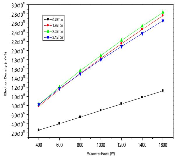
Fig-2. Dependence of electron density on microwave Power for different argon pressure at 19mm above the substrate
