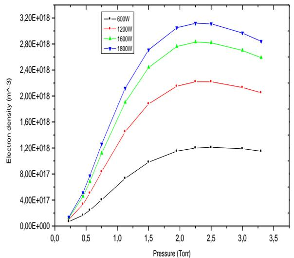
Fig-3. Dependence of electron density on argon pressure for different incident power at 19mm above the substrate
