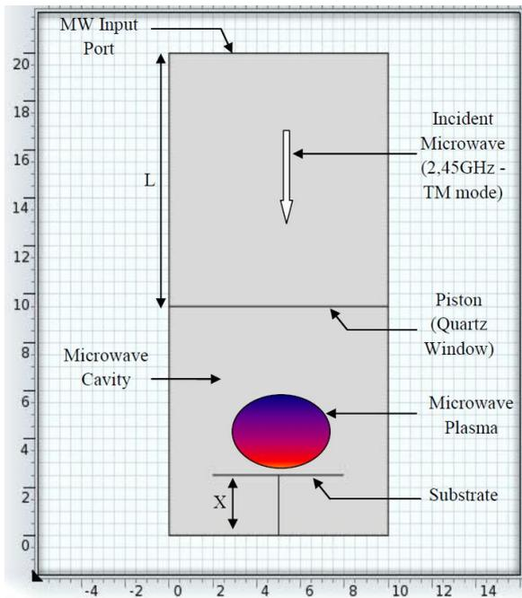
Fig-1. The diagram of 2D geometry modeled
