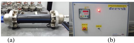
Figure 1. The used equipments (a) Closed pipe with end caps (b) Burst pressure control panel with a pressure sensor, pressure display and the pump control.
