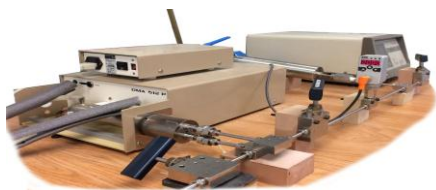
Figure 2. High pressure densimeter installation
