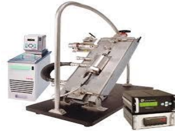
Figure 1. Viscometer (VISCOLab PVT) components The measurements obtained in function of the pressure show a linear behaviour for the density, dynamic viscosity, thermal expansion and mass expansion. Furthermore, the same component demonstrates the thermodiffusion coefficient.
