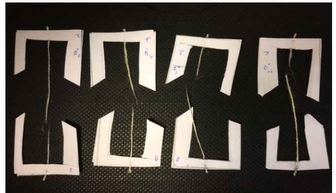
Fig 4. Hemp fibre yarn specimens after test
