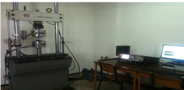
Figure 3. Machine MTS 810
