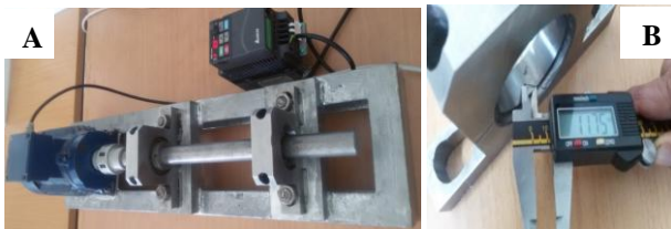
Fig. 1. (A) the experimental test bench, (B) artificial defect on the outer ring
